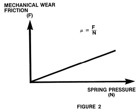
In addition to the coefficient of friction, it is also important to note that the mechanical wear will be influenced by speed at the interface of the sliding electrical contact. In fact, the rate of change in mechanical wear, or the slope of the graph, will change proportionately with either an increase or decrease of these two variables.
