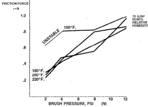
**GRAPH IA EFFECT OF PRESSURE ON COEFFICIENT OF FRICTION**
