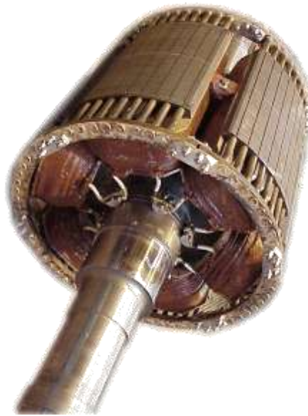
Slip Ring End [before slip-ring installation]
